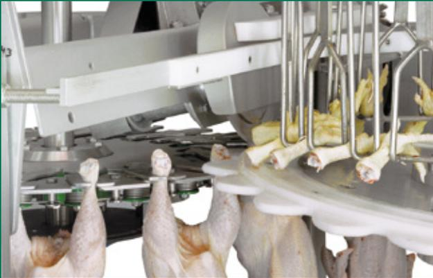
The Meyn hock cutter separates the hocks from the whole bird. The legs are positioned in a synthetic cutting wheel. When the shackle guide pushes the shackle inside, the ankle joints are bent. Depending on the setting of the machine, the rotating knife cuts through or below the ankle joint. The machine is placed in a corner wheel of the overhead conveyor of the slaughtering line or it can be integrated in the rehanger slaughtering/evisceration.
