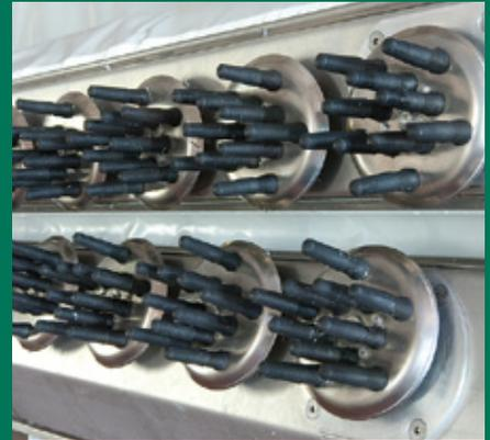
In the plucking line, the birds pass through a series of plucking machines that are equipped with motor driven rotating discs, each operating a number of plucking fingers. The discs closely follow the contours of the bird and water spray removes the plucked feathers. Easy and simple adjustment in height and width, even during production, provides excellent plucking results. Efficiency and ease of use are key features of Meyn's plucking equipment
