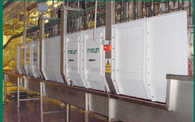
The electrical stimulator is part of Meyn's accelerated maturation concept. The use of electrical stimulation shortens the time post mortem that the product needs to reach rigor mortis, the state in which the product can be deboned. An off line chill room, needed for a long maturation before deboning, can be avoided, considerably reducing required floor space and handling cost.
