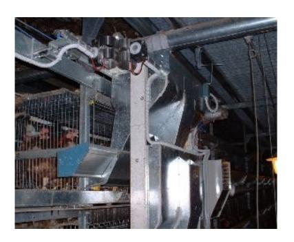
Egg belt blower for the lower section of the cages when the second floor is provided.
