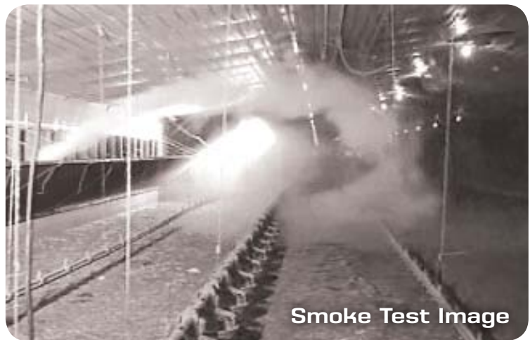
Air shoots upward and then swirls down and around from center of house for outstanding air mixing.
